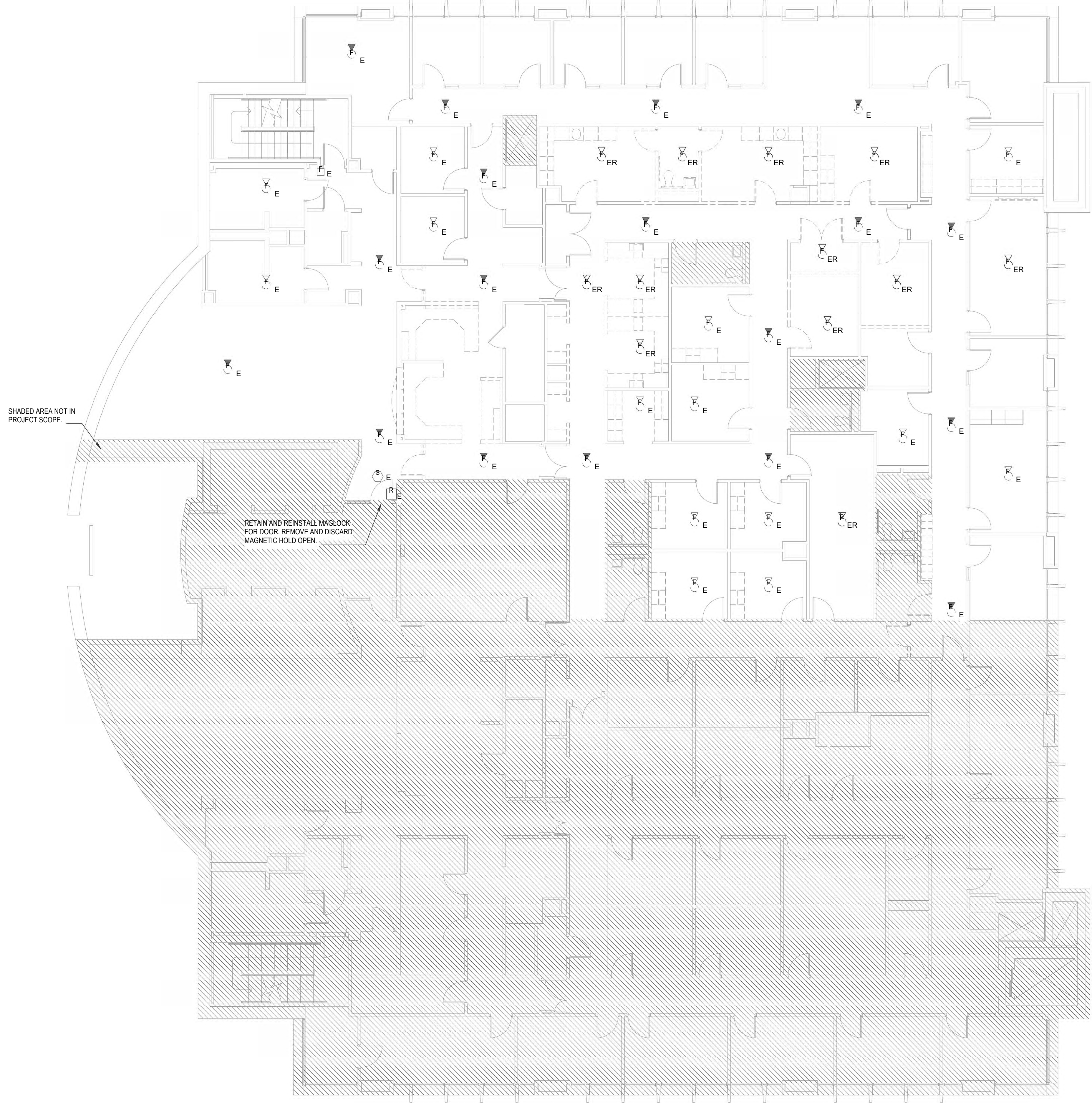
LEVEL 6 - FIRE ALARM DEMOLITION 1
